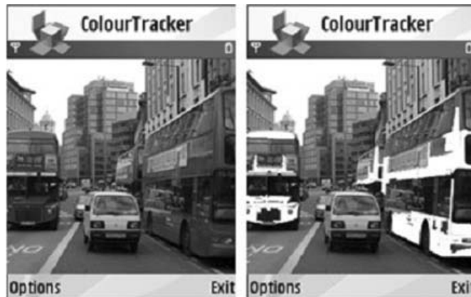
Figure 6.4 Screen shots of ColourTracker . The left image shows a red London Route Master bus before processing. The right image is after processing, where the red color has been identified, tracked and replaced with white
